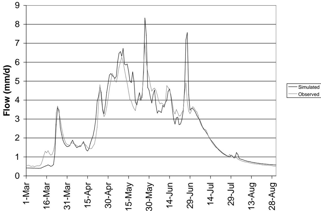
Figure 10. Observed, simulated streamflow for Boise River near Twin Springs, Idaho, 1998.
