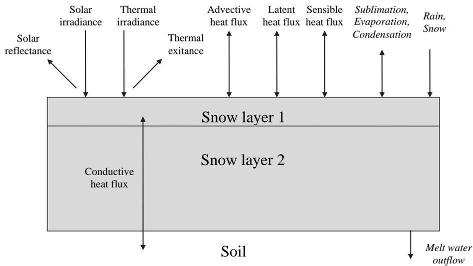
Figure 4. Diagram of ISNOBAL model components (energy fluxes in normal type, water fluxes in italics). Source: Garen and Marks (2005).
