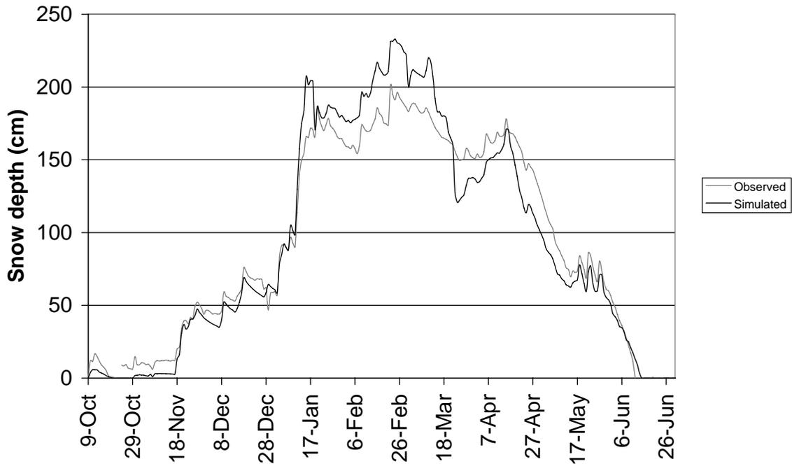
Figure 9. Observed, simulated (with ISNOBAL) snow depth for water year 1998 at Jackson Peak SNOTEL site (elevation 2,155 m), Boise River Basin, Idaho. Source: Garen and Marks, 2005.
