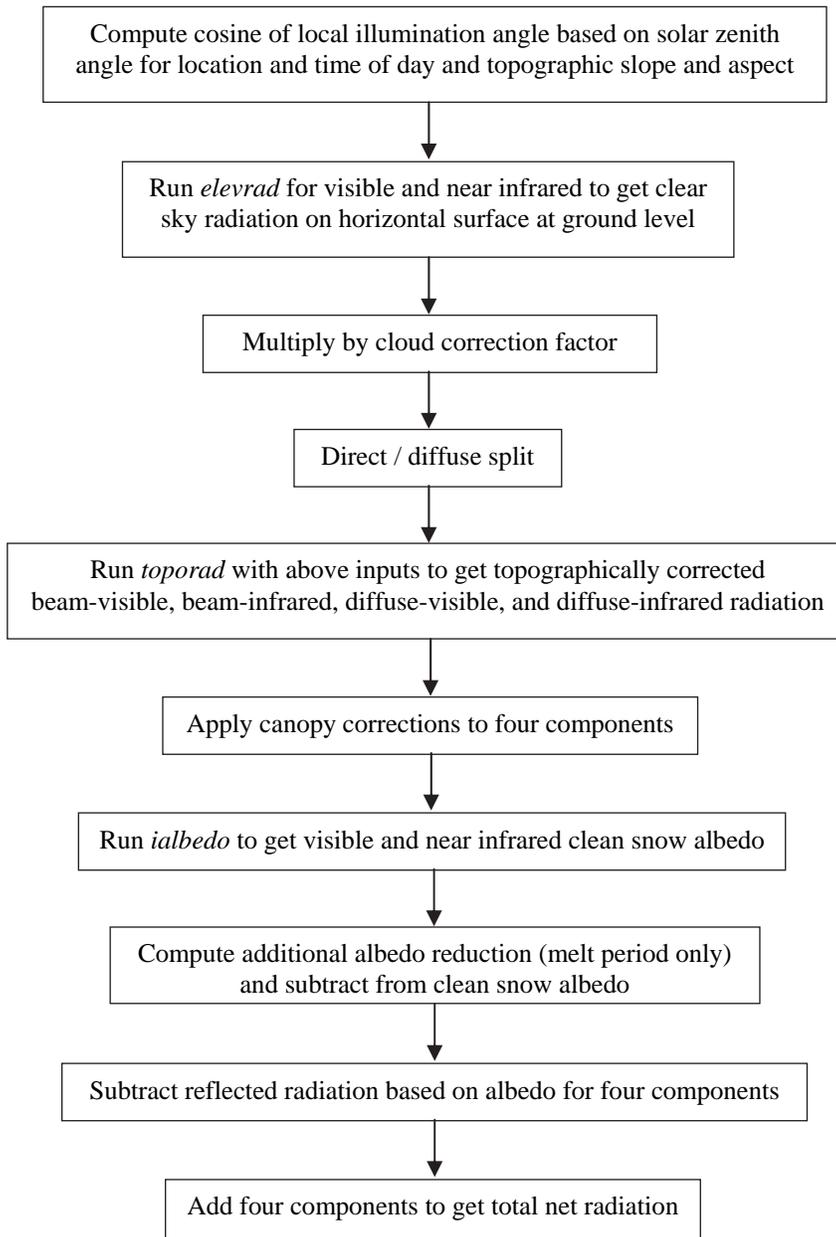
Figure 7. Flowchart of net radiation calculations for each 20-minute time step when the sun is up for each grid cell within the catchment (IPW utility names in italics). Source: Garen and Marks (2005).
