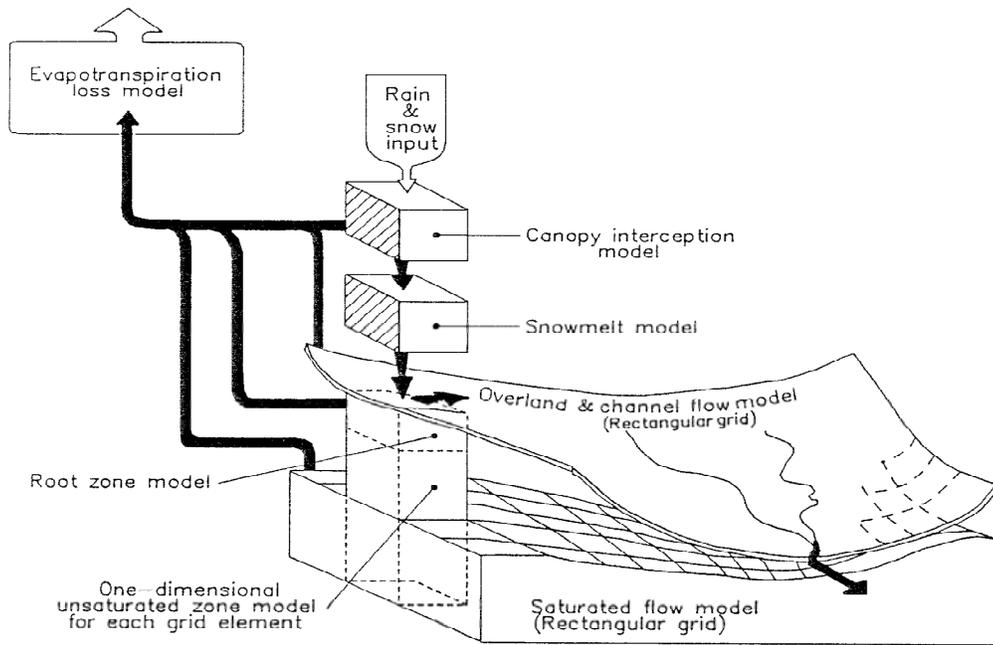
Figure 3. Schematic depiction of hydrologic processes represented in spatially distributed hydrologic modeling, many of the parameters of which are derived from basic and derived spatial data layers.
