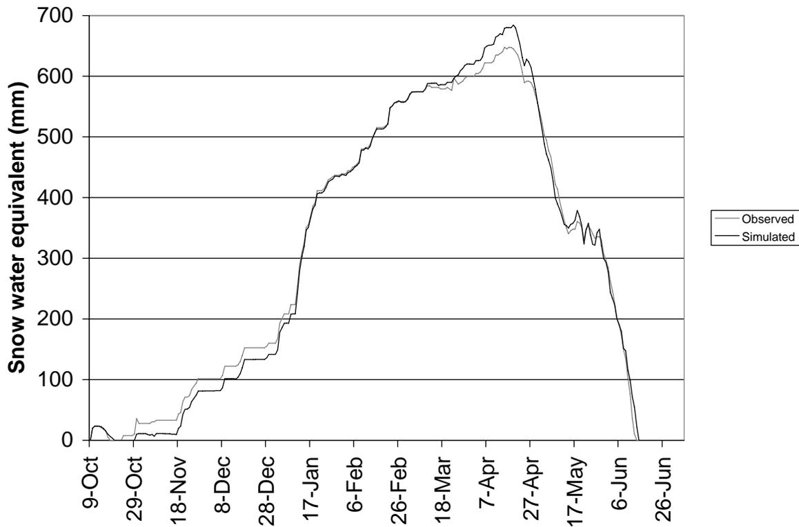
Figure 8. Observed, simulated (with ISNOBAL) snow water equivalent for water year 1998 at Jackson Peak SNOTEL site (elevation 2,155 m), Boise River Basin, Idaho. Source: Garen and Marks, 2005.
