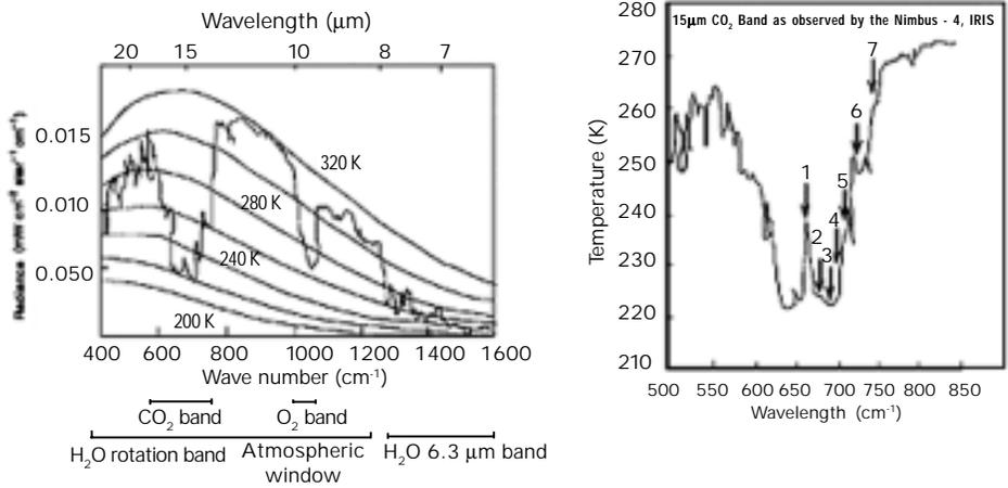
**Figure 3:** (a) Curve showing the absorption of infrared radiation by different gases in the atmosphere. (b) Numbers shown in this curve (1,2,3,4...7) denote the central wavelengths of CO<sub>2</sub> absorption band used for sounding of atmospheric temperature profiles
