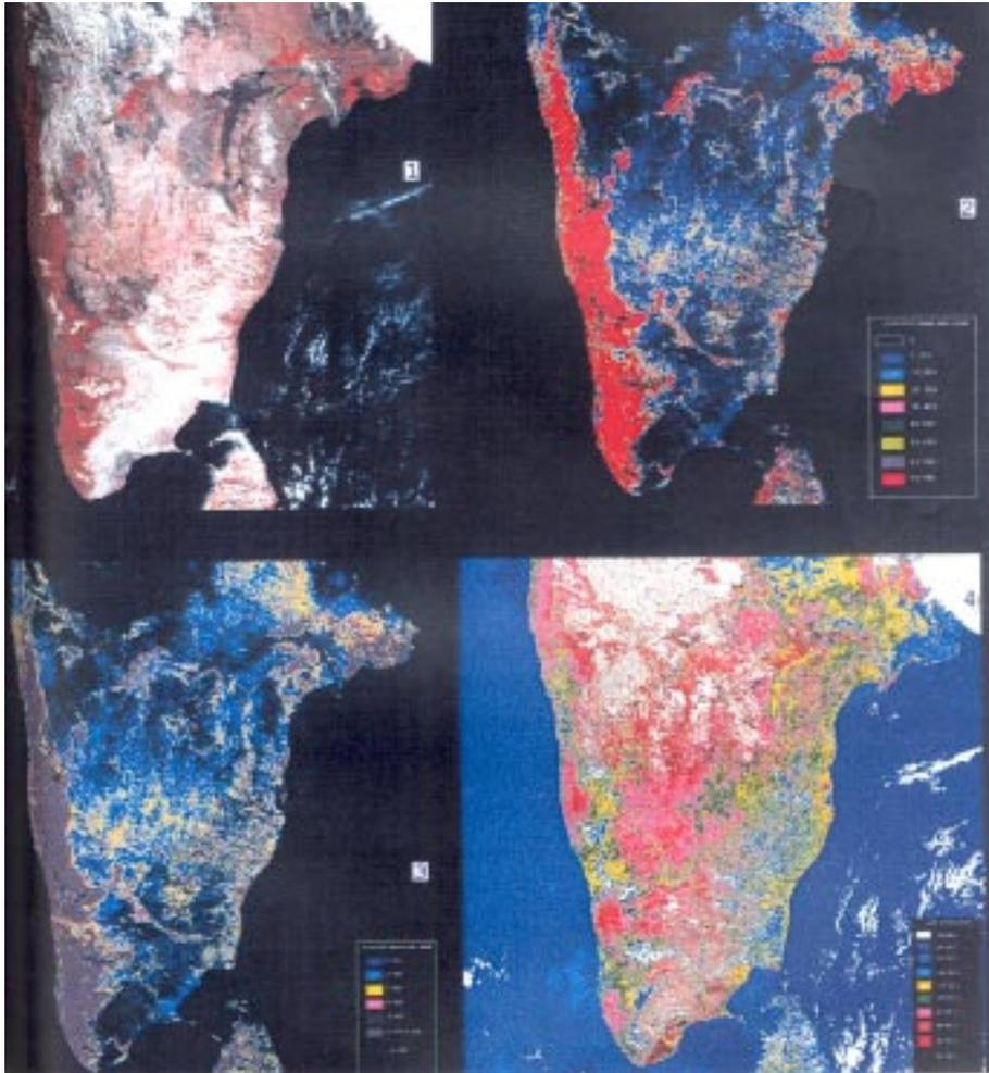
**Figure 5:** (1) FCC ( Ch2, Ch1, Ch1, R,G,B) ; (2) Vegetation proportion image; (3) Surface emissivity image and (4) Surface Temperature image - derived from processings of NOAA - AVHRR data ( southern India)
