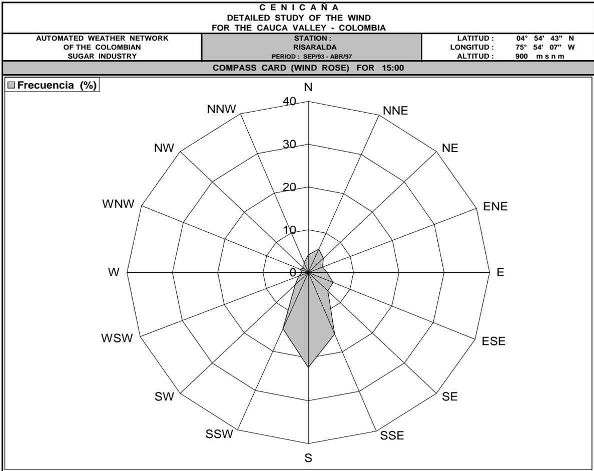
Figure 5. CENICAÑA – Automated weather network.
